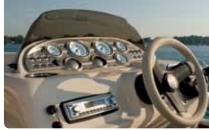
DRIVER'S CONSOLE Standard console features AM/FM stereo with a J-Port Private changing rooms add for MP3 players. Shown here with the gauge package.
