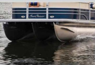
TUBES | Tubes are made with one-piece .080 gauge aluminum with full-length keels and sturdy deck risers. Backed by a Limited Lifetime Warranty.
