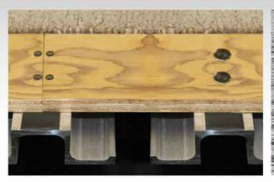
CONSTRUCTED FOR ENDURANCE I 3/4", 7-ply pressure treated plywood through-bolted and screwed to the stern hat channels to create the strongest seams and transom support in the industry.
