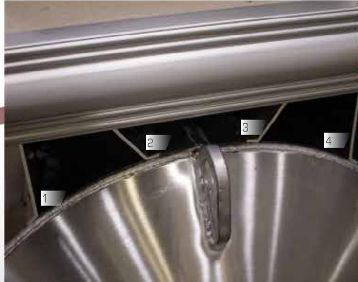
**4 POINT DECK TO HULL FUSION** | SunChaser deck brackets have 4 points of fusion for an extended area of contact with the tube. In addition to providing increased strength and support, this reduces frame twist and racking in rough water and guards against tube fatigue.
