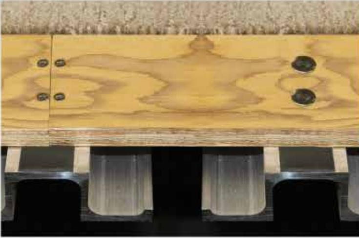
**CONSTRUCTED FOR ENDURANCE** | 3/4", 7-ply pressure treated plywood through-bolted and screwed to the stern hat channels to create the strongest seams and transom support in the industry.
