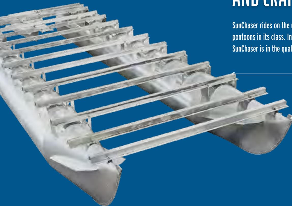
**CROSS CHANNEL CONSTRUCTION** Provides superior chassis strength. The transom area is supported with up to 3/16" hat-channel construction using twice the amount of fasteners as other pontoons. This provides the strength needed to handle the high torque of today's large engines.
