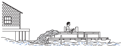
Blockage of boat exhaust by obstruction
